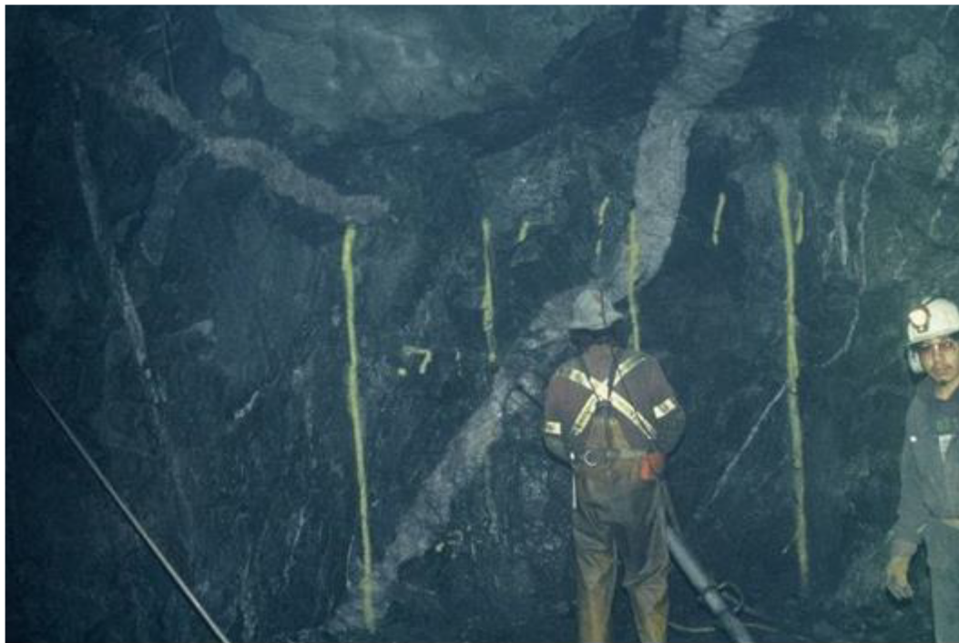
FIGURE 7.5 QUARTZ VEIN IN FACE AT THE 400 D SILL DRIFT
