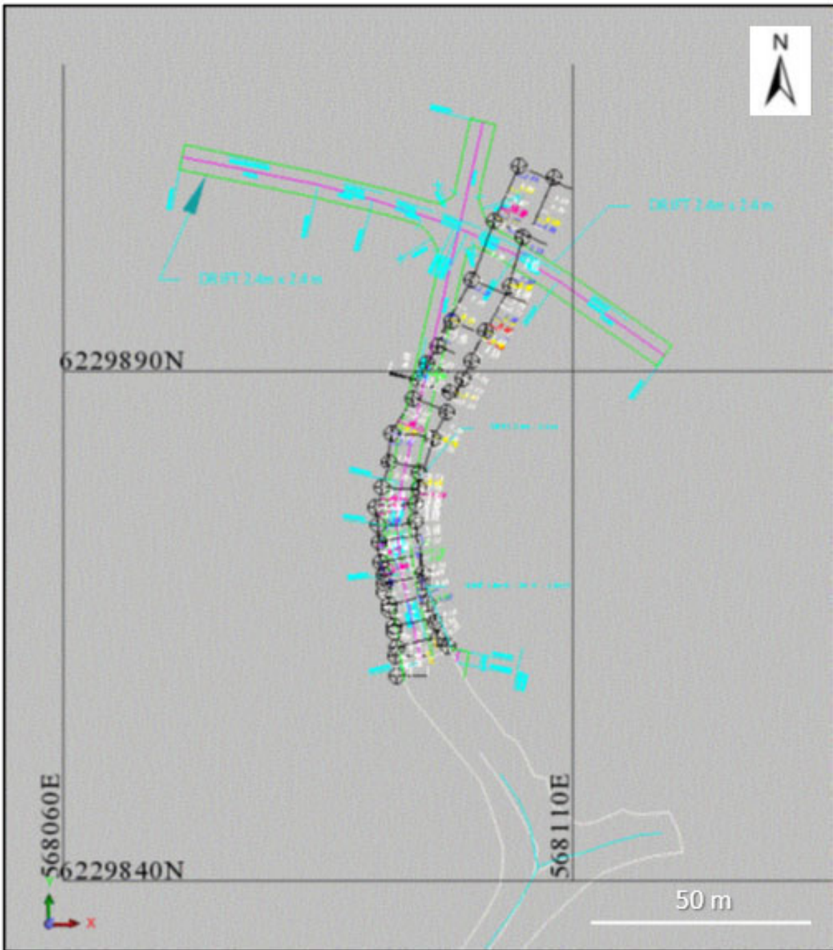
FIGURE 9.2 UNDERGROUND 300 LEVEL CROSS-CUT DEVELOPMENT
