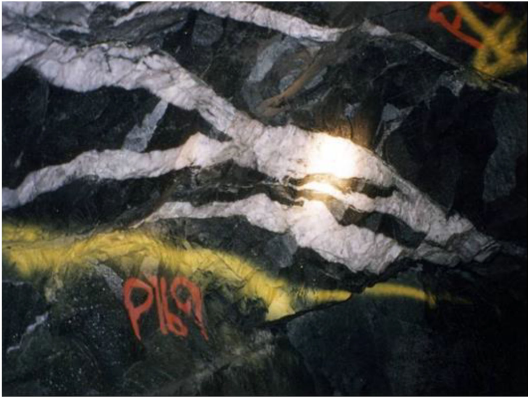
FIGURE 7.6 QUARTZ VEIN STRUCTURE ALONG THE BACK ON THE 400 D STOPE
