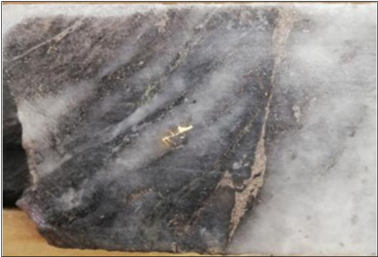
FIGURE 7.8 VISIBLE GOLD IN QUARTZ VEIN DRILL CORE SAMPLE FROM BINGO
